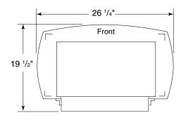
Figure 5 - Stove With Burner System Bottom Dimensions
